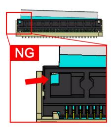
Detecting a part of the connected FPC/FFC indicates misinsertion
