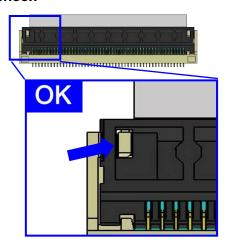
Detecting insulator of the connector indicates full insertion
